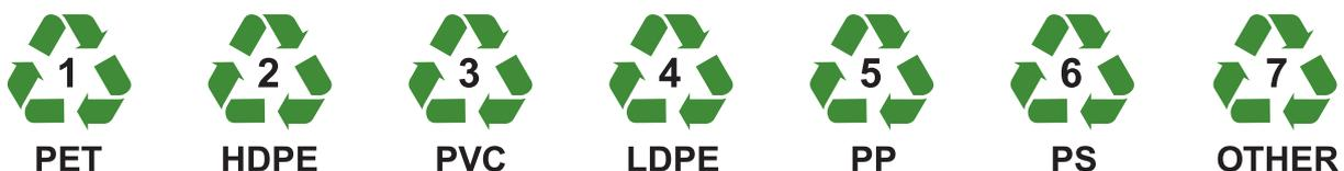
This international coding system was developed to provide manufacturers and recyclers' with a uniform identification system. Using this resin identification code enables recyclers to sort plastic into each resin type thereby producing a quality recyclate commodity. The Plastics Identification Code does not equal recyclability as is commonly assumed. It assists consumers to correctly identify which plastics are acceptable in municipal recycling collections and which are not.
