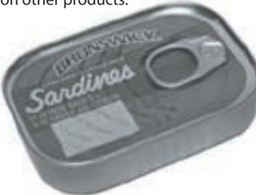
Providing a key to open a can along a scored line is common for meat products likely to be eaten in conditions where a can opener may not be available. In the example below, the can is tapered and, after opening with the key, the top can be easily lifted off to leave the product on the can base for serving.
