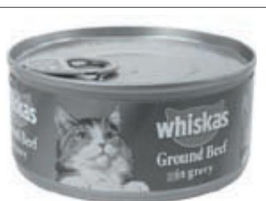
The pet food industry is a major user of metal cans. The photograph shows a two piece steel can with a pull-tab end. The can body is drawn from one piece of metal. Heat processing produces a lower-than-atmospheric pressure within the can.
