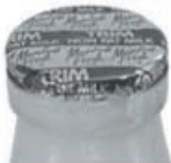
An aluminium foil top on a glass bottle of milk. The foil can be shaped and placed by machine on the bottle and is economical in cost and in materials. It does not react with the milk, is impermeable, easy to open, and provides tamper evidence.
